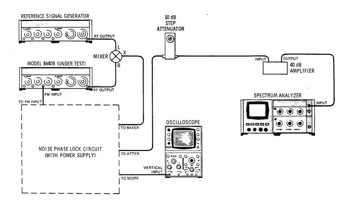
Figure 4-6. Single Sideband Phase Noise Test Setup
