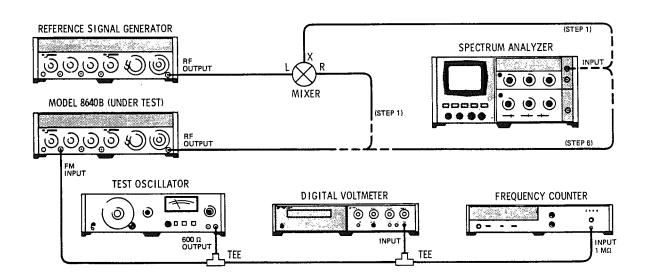
Figure 4-26. FM Sensitivity and Accuracy Test Setup
