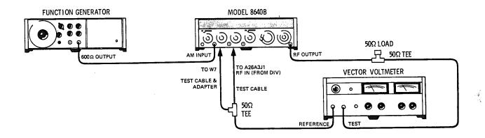
Figure 4-21. Peak Incidental Phase Modulation Test Setup
