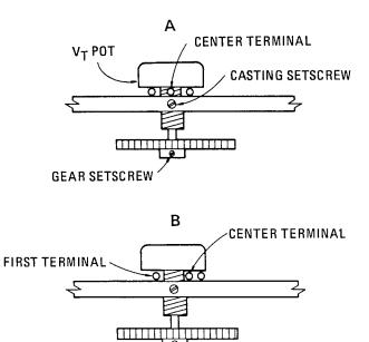
Figure 5-3. V<sub>T</sub> Pot Adjustment
