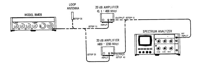
Figure 4-15. Output Leakage Test Setup
