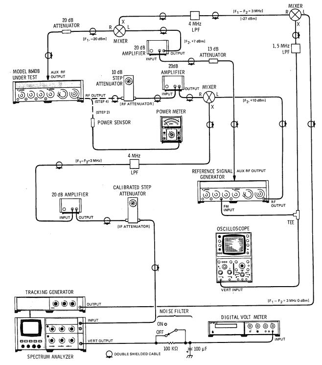
Figure 4-11. Output Level Accuracy Test Setup (Complete)
