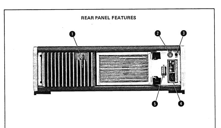
AUX RF OUT: nominal -5 dBm auxiliary RF output; 500 ohm source impedance. Signal does not contain amplitude or pulse modulation (however, it does contain FM). On the 512-1024 MHz/Doubler Band the auxiliary RF output is one-half the frequency of the indicated RF frequency.
