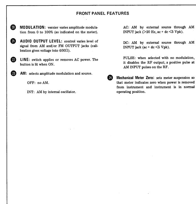
Figure 3-2. Front Panel Controls, Indicators, and Connectors (4 of 4)
