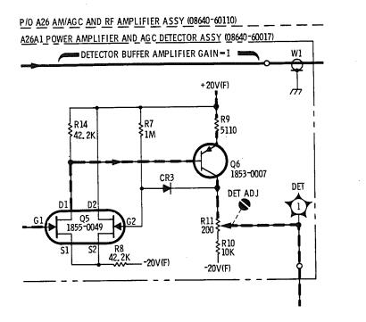
Figure 7-3. A26A1 Power Amplifier and AGC Detector Assembly Backdating (Change D)
