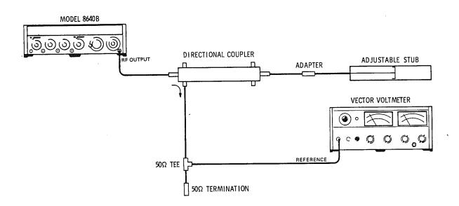
Figure 4-13. Output Impedance Test Setup (In Band)
