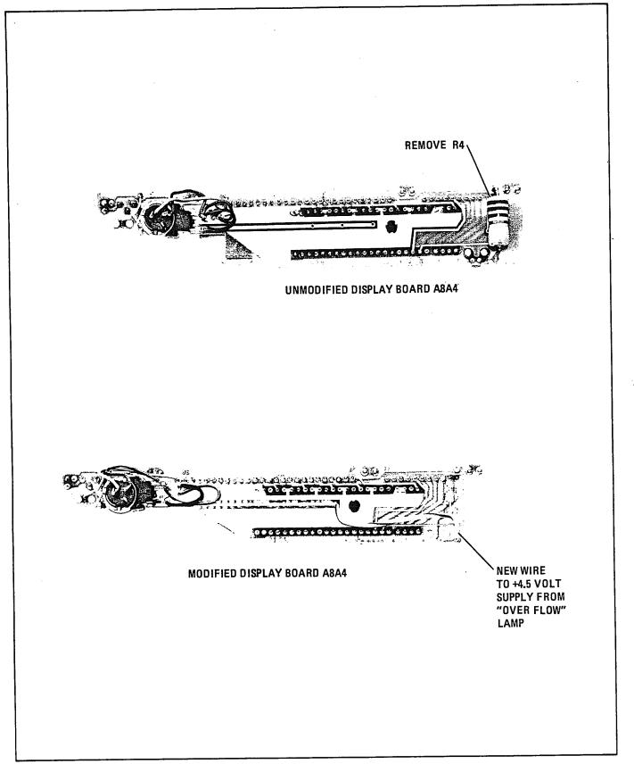
Figure 7-8. A8A4 Counter Display Assembly Modification
