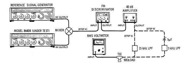
Figure 4-9. Residual FM Test Setup
