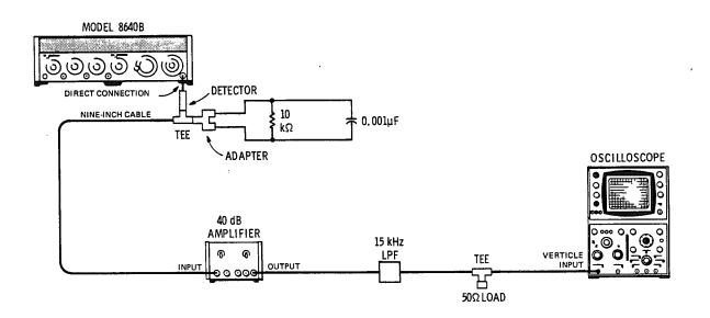
Figure 4-27. Incidental AM Test Setup
