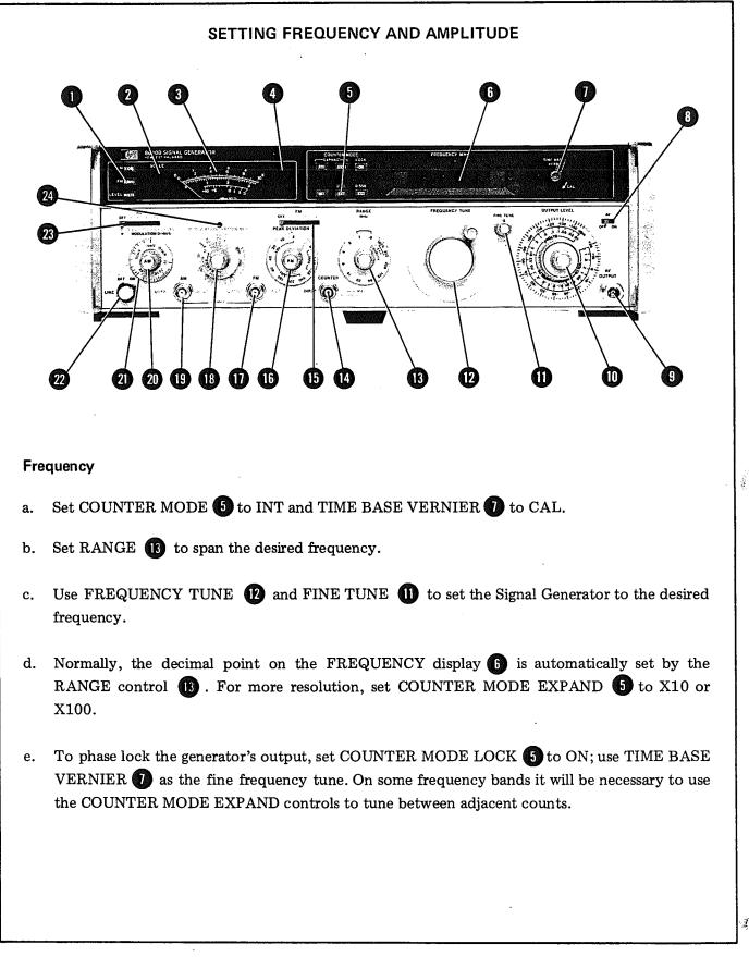
Figure 3-5. Setting the Frequency and Amplitude Controls (1 of 3)
