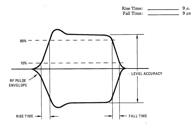
Figure 4-23. Pulse Measurements
