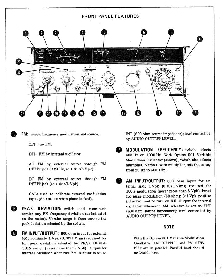
Figure 3-2. Front Panel Controls, Indicators, and Connectors (3 of 4)
