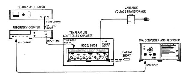
Figure 4-30. Internal Reference Drift Rate (Stability) Test Setup
