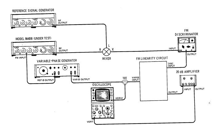
Figure 5-7. FM Linearity Adjustment Test Setup
