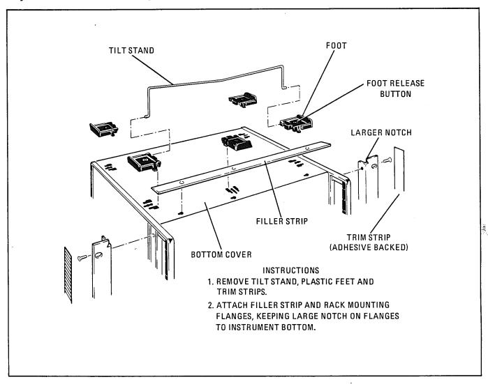
Figure 2-3. Preparation for Rack Mounting
