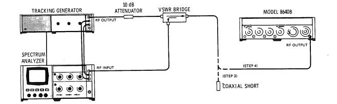
Figure 4-14. Output Impedance Test Setup (Out of Band)
