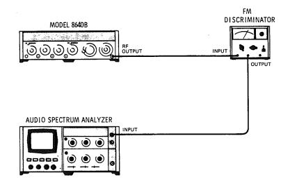
Figure 4-25. FM Distortion Test Setup
