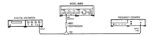
Figure 4-16. Internal Modulation Oscillator Test Setup
