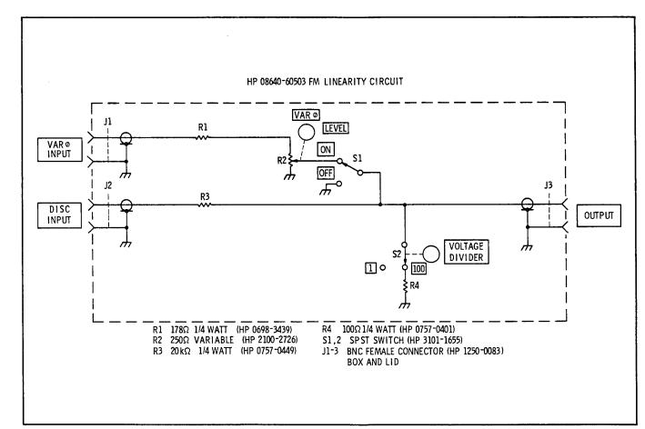
Figure 1-8. FM Linearity Circuit
