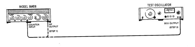
Figure 4-28. Counter External Sensitivity Test Setup
