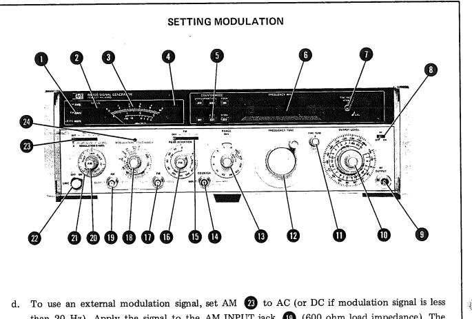
than 20 Hz). Apply the signal to the AM INPUT jack (19) (600 ohm load impedance). The Signal Generator requires 1 Vpk (0.7071 Vrms) for 100% modulation. Set percent of modulation with the MODULATION vernier (20); modulation % is indicated by the meter (3).
