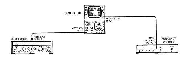
Figure 5-10. Internal Reference Frequency Adjustment Test Setup
