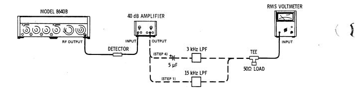
Figure 4-8. Residual AM Test Setup
