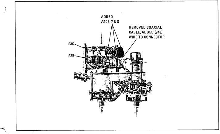
Figure 7-10. A9 Peak Deviation and Range Switch Modification
