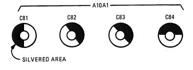
Figure 5-6. 256-512 MHz High Band Capacitor Adjustment Orientation
