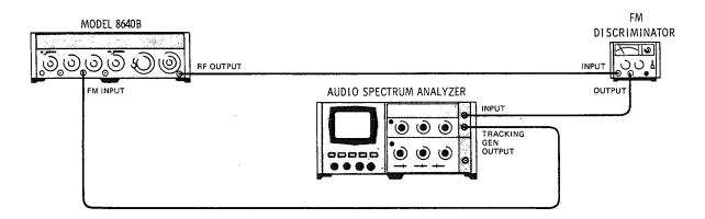
Figure 4-24. FM 3 dB Bandwidth Test Setup
