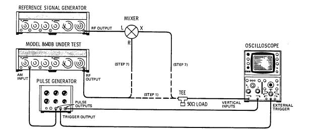
Figure 4-22. Pulse Modulation Test Setup
