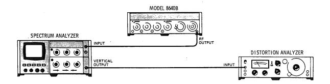
Figure 4-19. AM Distortion Test Setup
