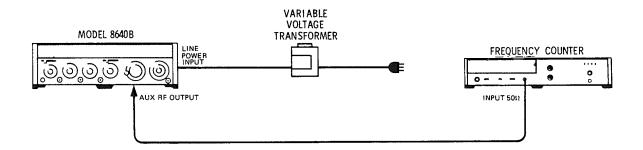
Figure 4-3. Frequency Stability vs Line Voltage Test Setup
