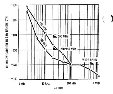
Figure 1-2. Measured Single Sideband Noise vs Offset from Carrier. (Stated in a 1 Hz Bandwidth at 256 and 512 MHz Carrier Frequencies on 256 - 512 MHz Band.) Markers indicate specified limits.
