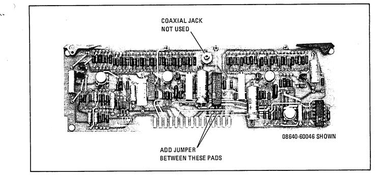
Figure 7-9. A7 FM Shaping Assembly Modification
