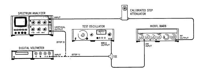
Figure 4-20. AM Sensitivity and Accuracy Test Setup
